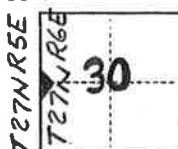
CORNER — LEFT AS FOUND  FOUND AND TAGGED  REESTABLISHED OBLITERATED CORNER  REBUILT
