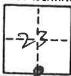
Sept. 11 1997CORNER — LEFT AS FOUND FOUND AND TAGGED REESTABLISHED OBLITERATED CORNER REBUILT
