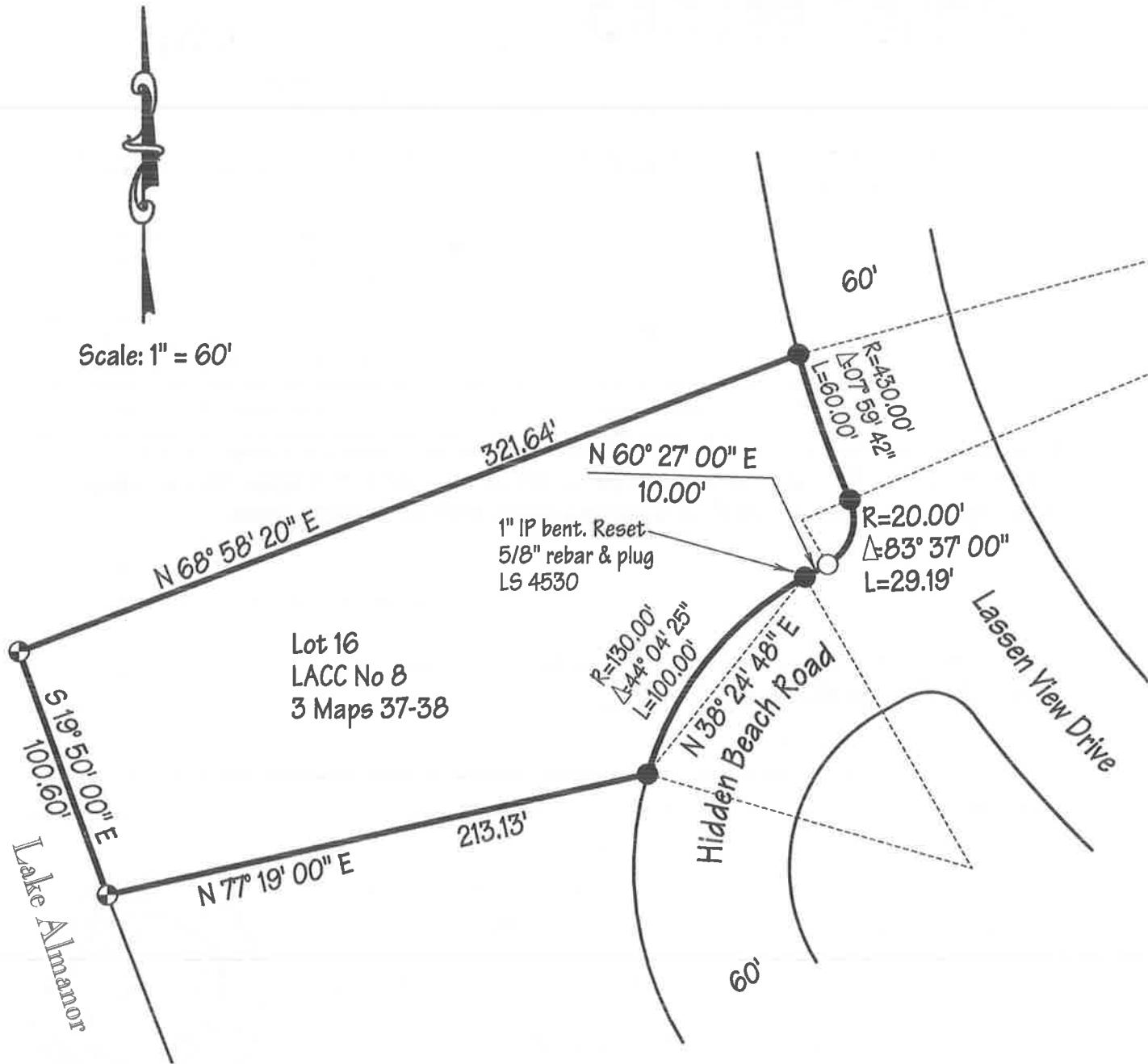
Basis of Bearings: The chord bearing between the 2 found monuments on the 130' radius curve being N 38° 24' 48" E calculated from record per 3 Maps 38.
