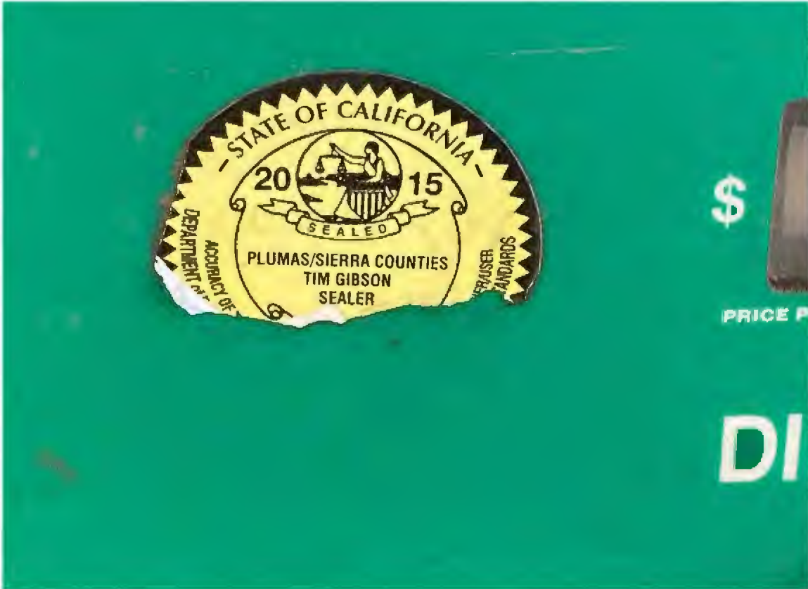
Figure 3 - Fuel pump last inspected in 2015 which is 4 years out of inspection compliance.
