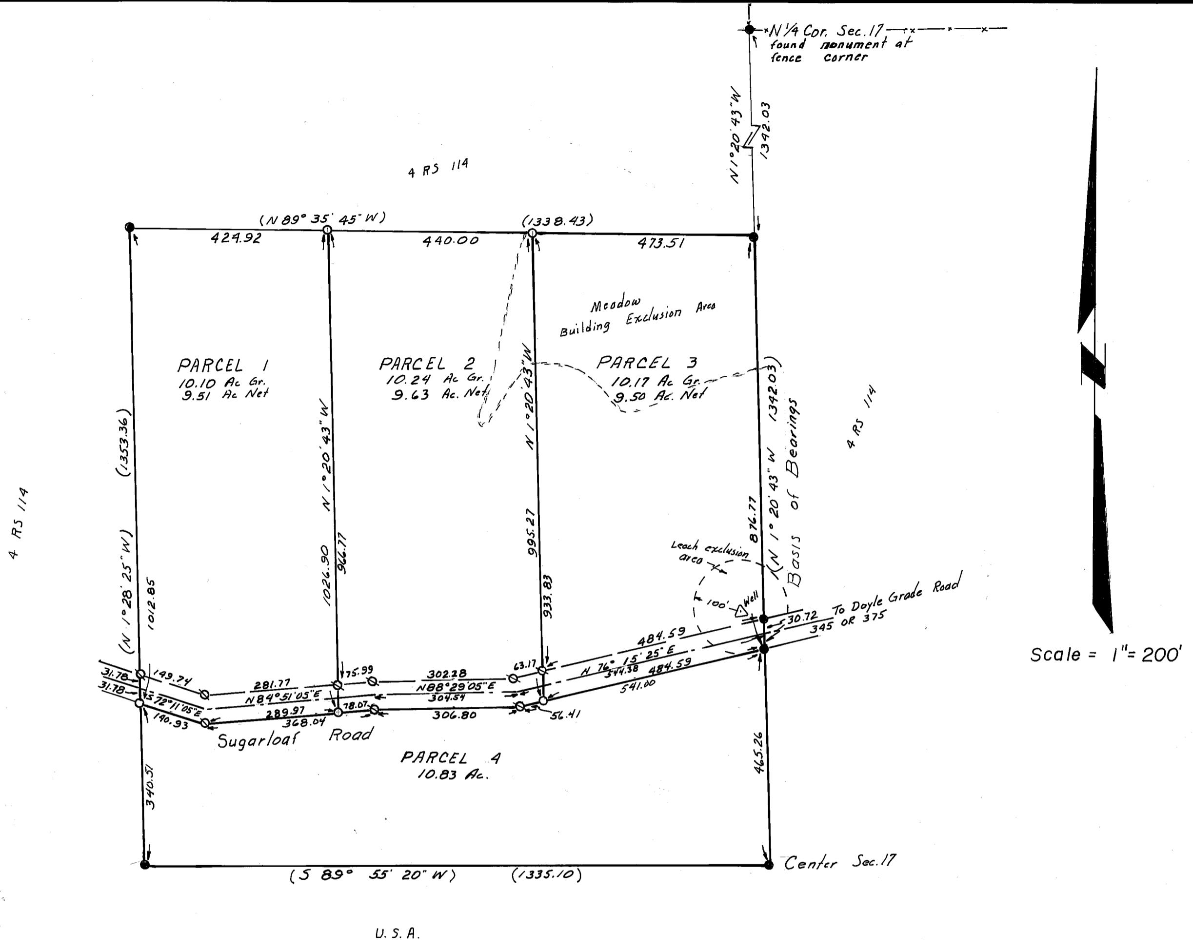
The BASIS OF BEARINGS is the west line of the N.E. 1/4 of Section 17, shown as  $N 1^{\circ} 20' 43'' W$  on 4 R.S. 114.
