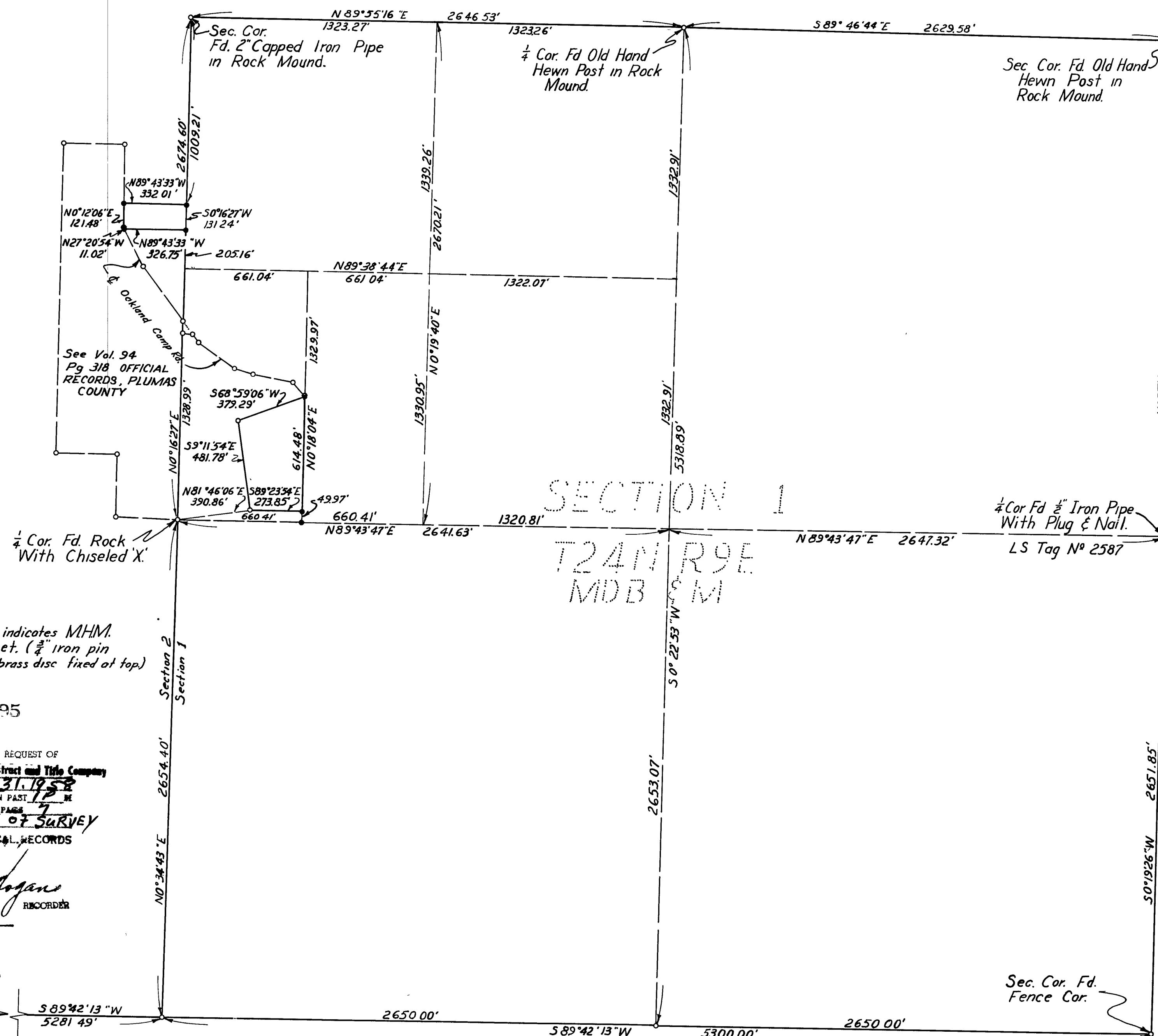
I, Leonard E. Bowser, do hereby certify that I am a Licensed Land Surveyor of the State of California, that the map delineated hereon correctly represents a survey made by me in April 1958 and all monuments shown hereon are of the character and occupy the positions indicated and are sufficient to enable the survey to be retraced.
