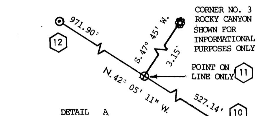
SET: A STANDARD U.S.F.S. MONUMENT 22 INS. IN THE GROUND AS "POINT ON LINE ONLY", NO STONE MOUND CONSTRUCTED. NOTHING SET AT CORNER NO. 3, ROCKY CANYON LODE.
