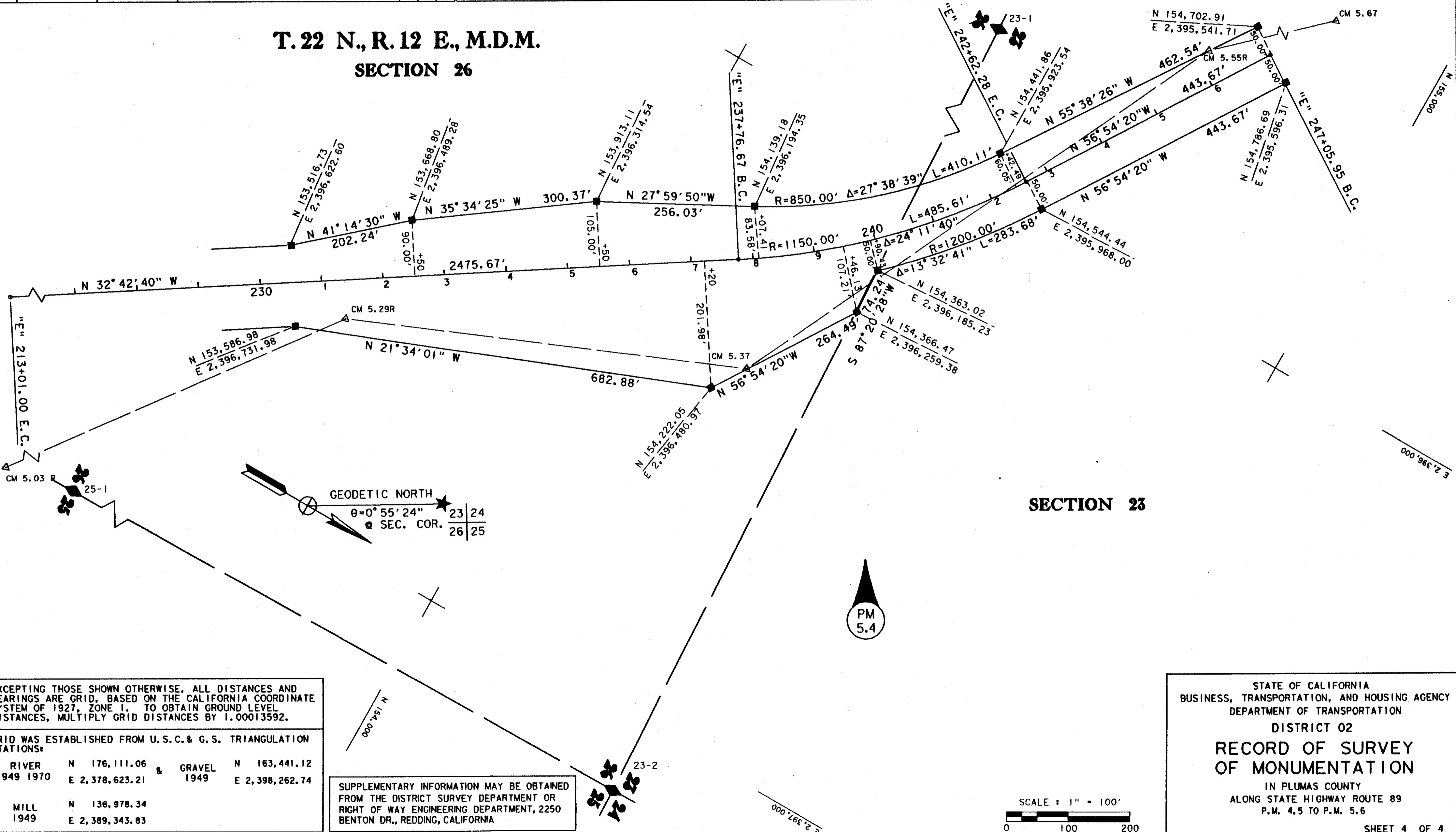
EXCEPTING THOSE SHOWN OTHERWISE, ALL DISTANCES AND BEARINGS ARE GRID, BASED ON THE CALIFORNIA COORDINATE SYSTEM OF 1927, ZONE I. TO OBTAIN GROUND LEVEL DISTANCES, MULTIPLY GRID DISTANCES BY 1.00013592.
