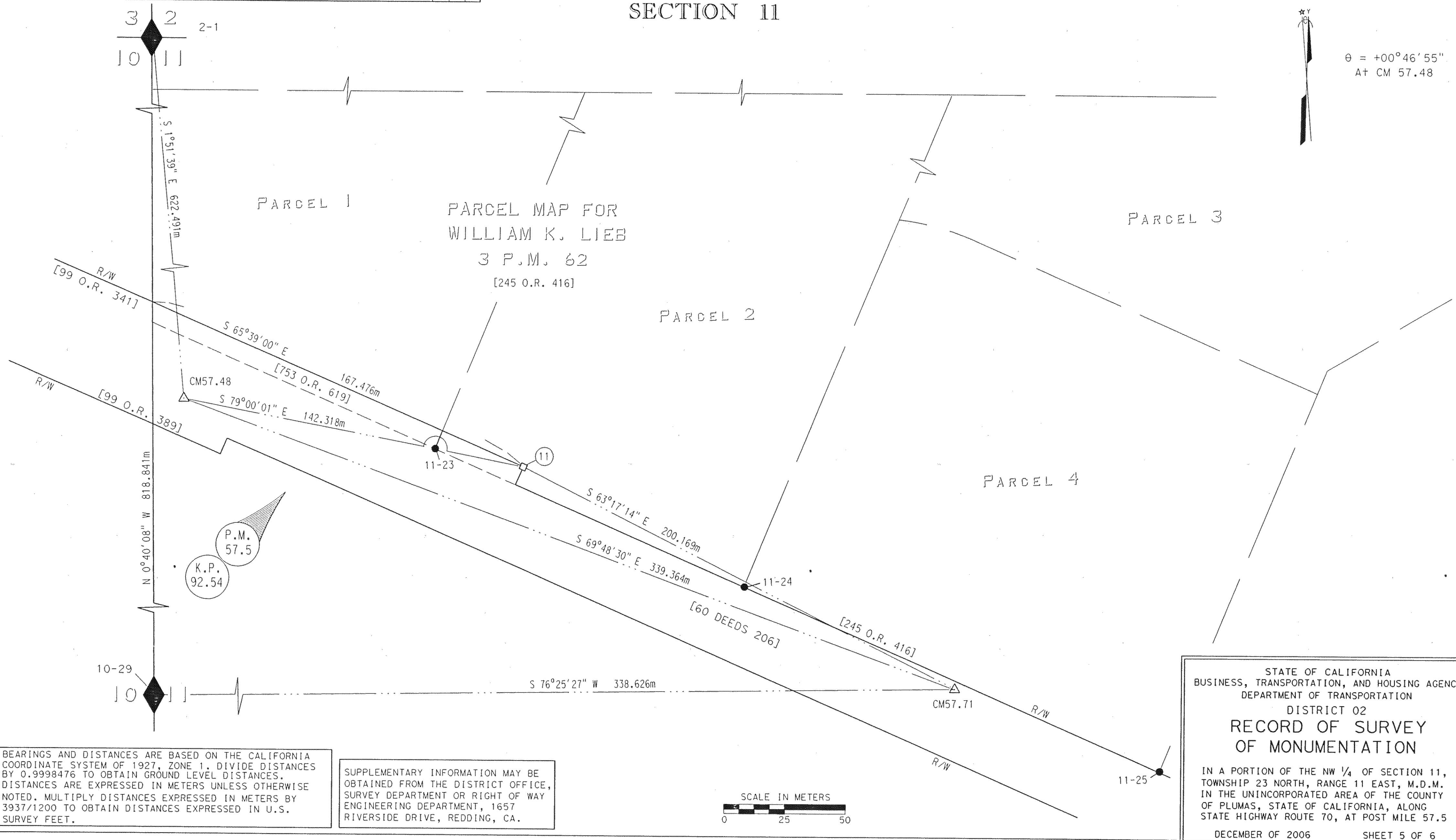
BEARINGS AND DISTANCES ARE BASED ON THE CALIFORNIA COORDINATE SYSTEM OF 1927, ZONE 1. DIVIDE DISTANCES BY 0.9998476 TO OBTAIN GROUND LEVEL DISTANCES. DISTANCES ARE EXPRESSED IN METERS UNLESS OTHERWISE NOTED. MULTIPLY DISTANCES EXPRESSED IN METERS BY 3937/1200 TO OBTAIN DISTANCES EXPRESSED IN U.S. SURVEY FEET.
