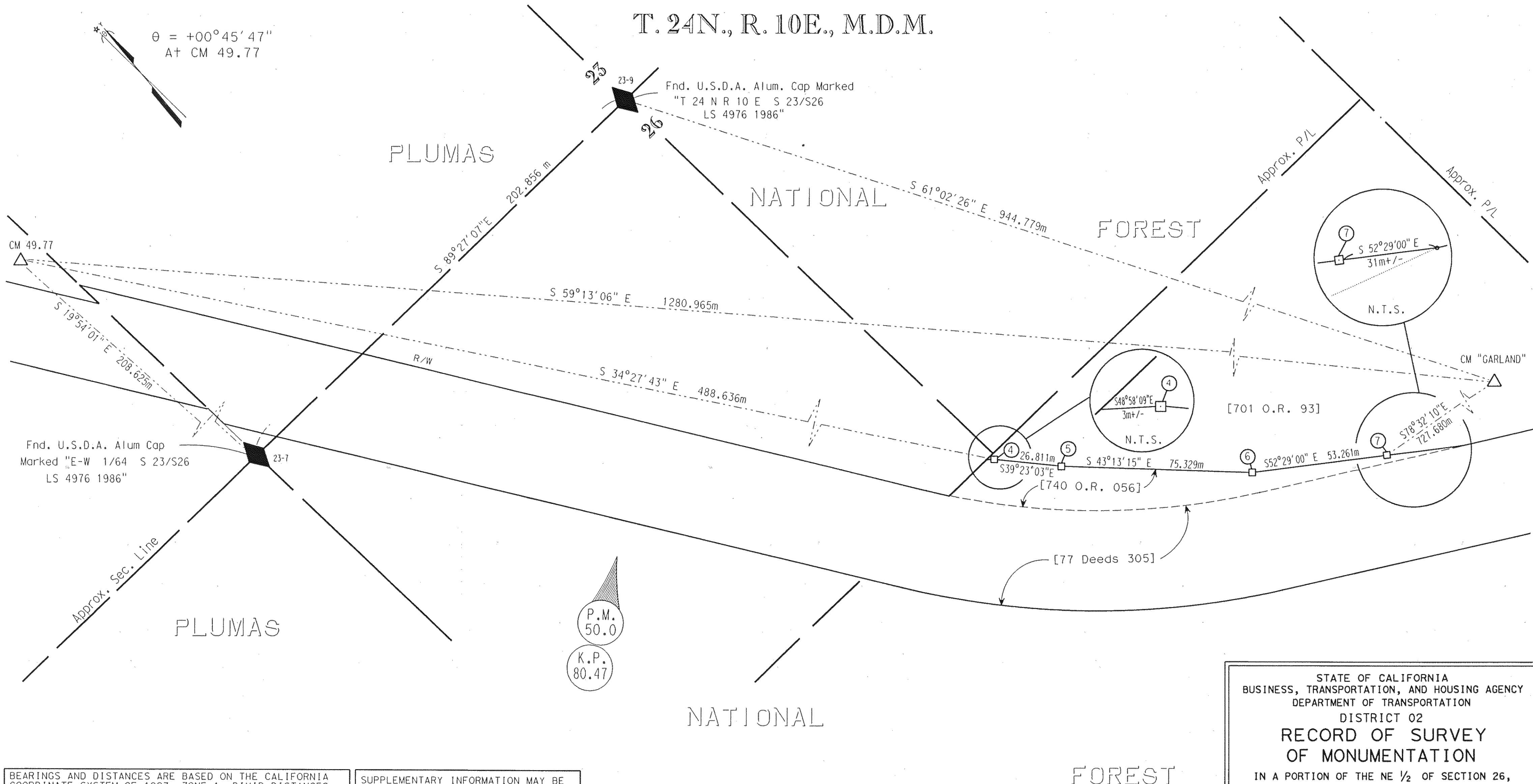
BEARINGS AND DISTANCES ARE BASED ON THE CALIFORNIA COORDINATE SYSTEM OF 1927, ZONE 1. DIVIDE DISTANCES BY 0.9998476 TO OBTAIN GROUND LEVEL DISTANCES. DISTANCES ARE EXPRESSED IN METERS UNLESS OTHERWISE NOTED. MULTIPLY DISTANCES EXPRESSED IN METERS BY 3937/1200 TO OBTAIN DISTANCES EXPRESSED IN U.S. SURVEY FEET.
