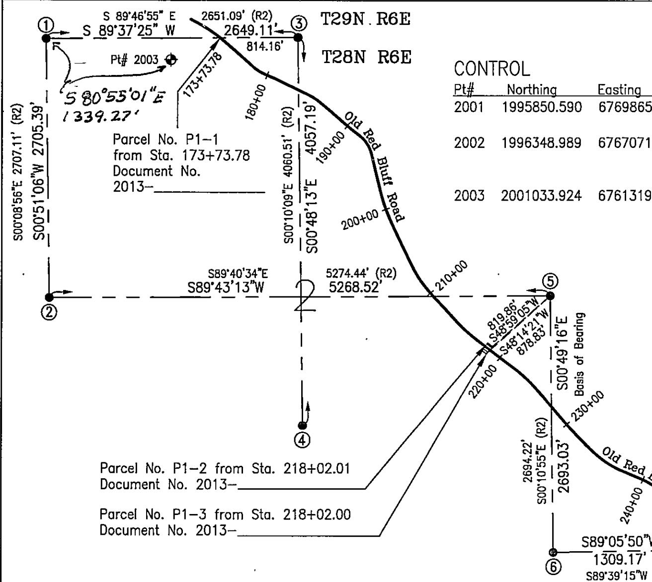
1) Fd. 3 1/4" Brass Cap stamped "U.S.DEP.T. OF THE INTERIOR BUR. OF LAND MANAGEMENT UNLAWFUL TO DISTURB T29N R6E S34 S35 S3 S2 T28N 1973 CADASTRAL SURVEY" on 1 1/2" Iron Pipe in a ring of stones accepted as the Northwest Corner Section 2: Shown on 4 R/S 101
