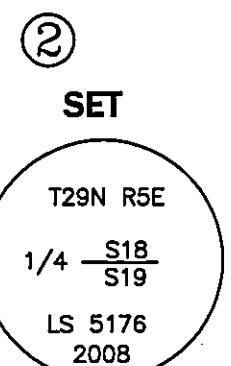
No original evidence found. At single proportion position, set a Standard USDA Monument 10" above ground in a 2' dia. by 11" high stone mound. From which bears (new):
