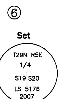
No original evidence found. At single proportion position, set a Standard USDA Monument 8" above ground in a 2' dia. stone mound. From which bears (new):
